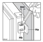
Open the appliance door and the furniture door at 90°. Insert the small square (Hb) into guide (Ha). Put together the appliance door and the furniture door and mark the holes as indicated in the figure.
